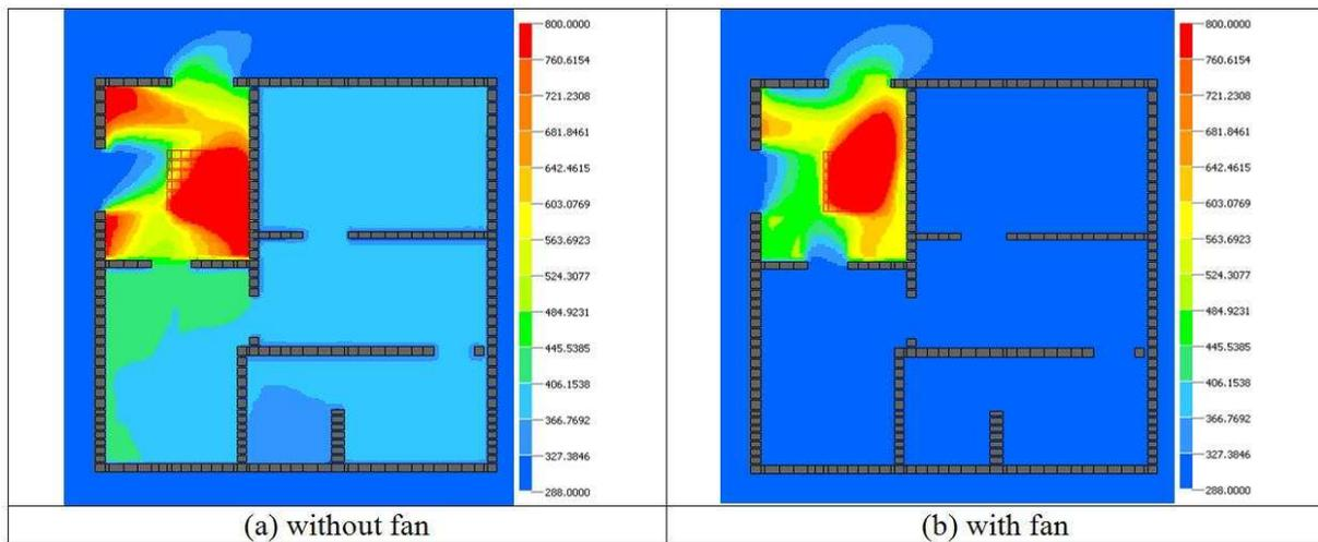
Figure 12 Smoke mass fraction along stairwell vertical plane (350 sec)
