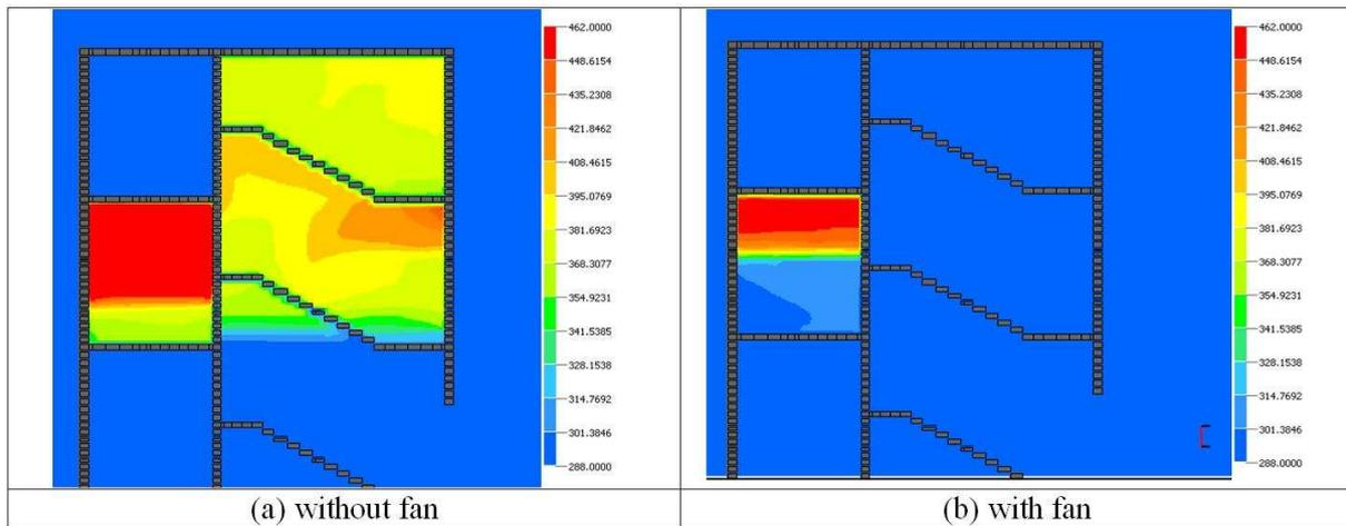
Figure 11 Temperatures (K) across the first floor layout at 1.22 m height (350 sec)
