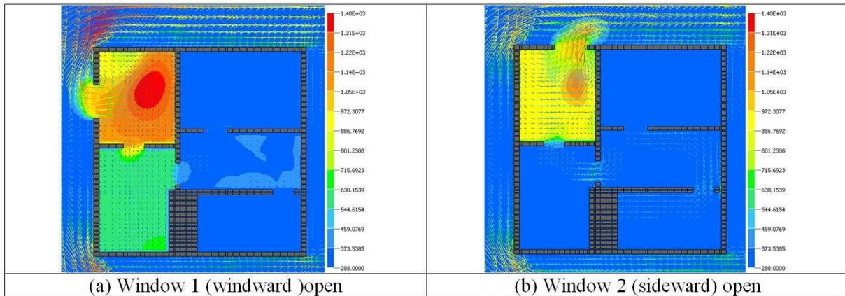
Figures 16a and 17a show that the smoke fills all the rooms of the fire apartment and also the stairwell region above the first floor which might put the occupants of fire apartment and the floors above at risk. It will also make the search and rescue operations difficult for the fire fighters. Figures 16b and 17b demonstrate that the PPV fan is able to contain the smoke within the room of fire origin and maintain better visibility in the stairwell area.
