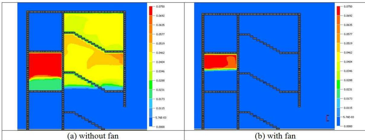
Figure 13 Smoke mass fraction across the first floor layout at 1.22 m height (350 sec)
