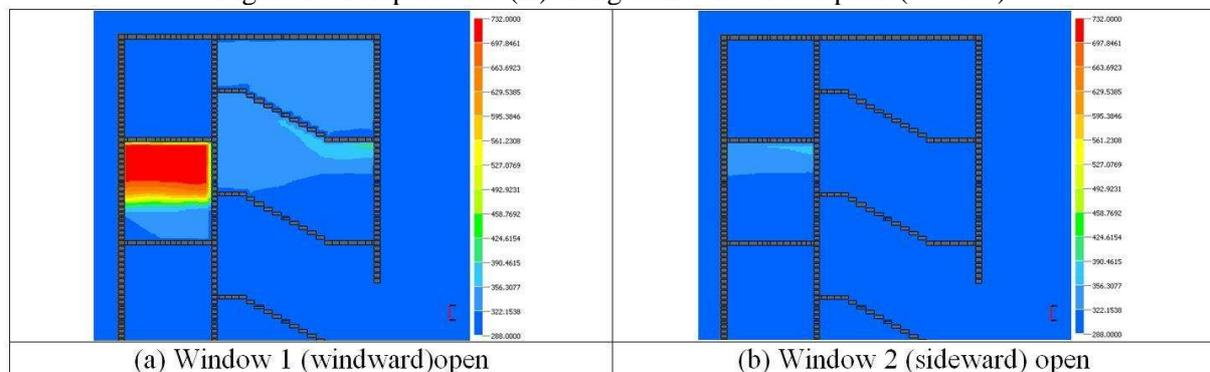
Figure 15 Temperatures (K) across the first floor layout at 1.22 m height (350 sec)
