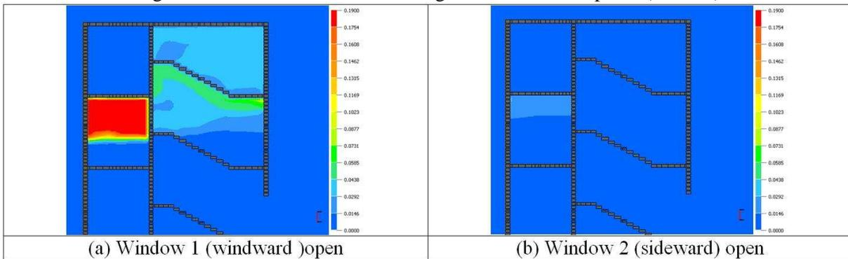
Figure 17 Smoke mass fraction across the first floor layout at 1.22 m height (350 sec)
