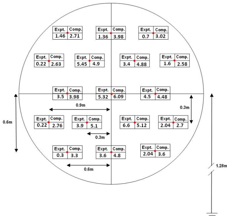
Figure 3 Horizontal velocity comparisons on a vertical plane at 3.05 m from fan outlet
